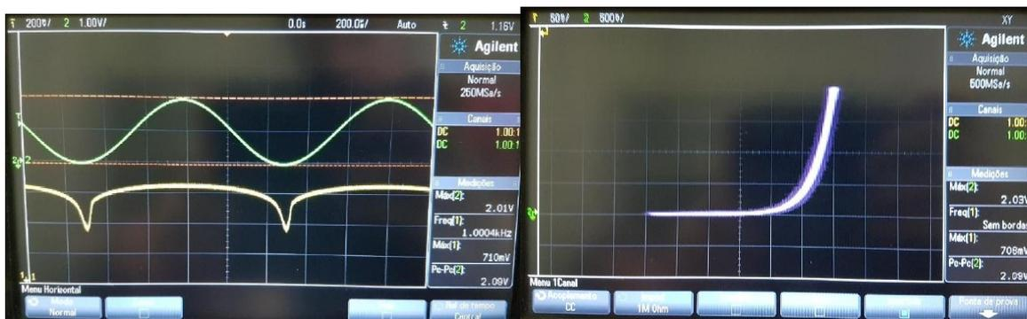
**Figura 8:**  $I_c$  versus  $V_{BE}$
