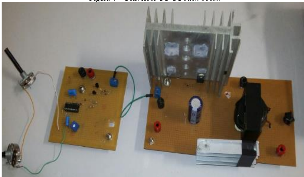
Figura 4 – Conversor CC-CC buck-boost .
