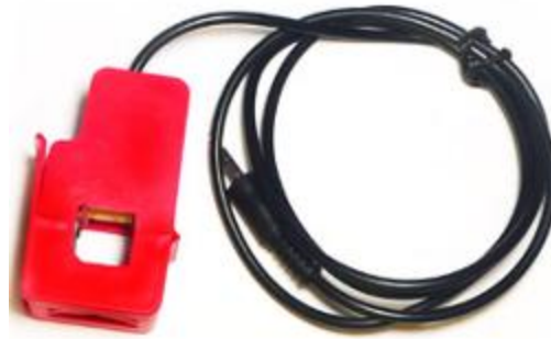
Figura 2 - Sensor transformador de corrente (NON-INVASIVE AC CURRENT...,2010)
