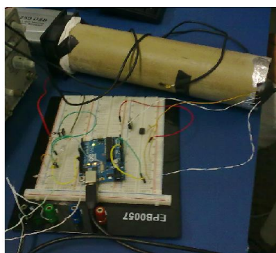
(a) Detalhe do kit Arduino e Drivers.
